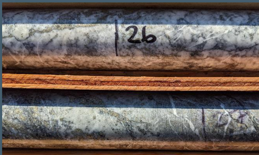
KH21-45 @ 26m: Gold-bearing Quartz-carb-sulphide veins
